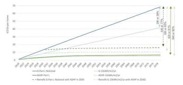
Figure 3-1. Comparison of cumulative CO<sub>2</sub> emissions from a house built to different energy performance standards. Source: CCC (2019)
