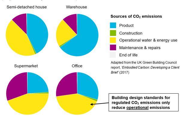
Figure 3-2. Illustration showing the relative proportion of CO<sub>2</sub> emissions from operational carbon (in yellow) compared with embodied carbon over a 30-year period. Source: UK-GBC (2017)
