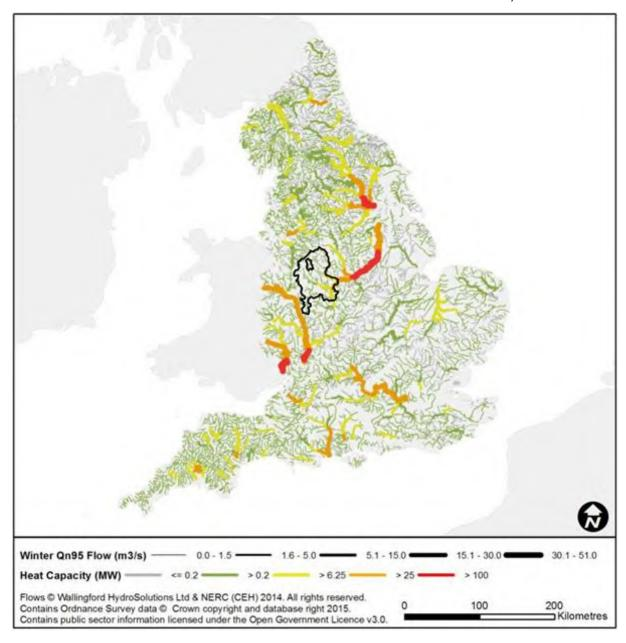
Figure 4-2. River heat capacity. Source: DECC (2015)
