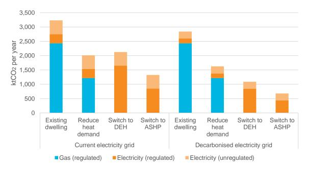
Figure 3-3. Estimated CO<sub>2</sub> savings that could be achieved in typical dwellings – based on different scenarios for regulated CO<sub>2</sub> emissions, heating system and electricity grid decarbonisation
