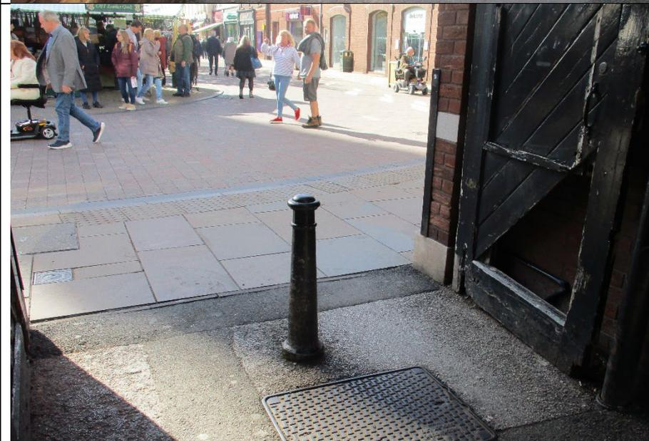
The bollard at the end of the footpath which is well placed but would benefit from some contrast in poorer light conditions.
