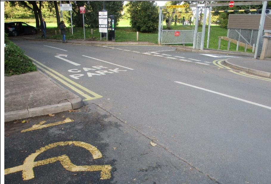
The end of the Blue Badge Bay showing that a person unloading a mobility aid from the rear of a vehicle would be in the path of traffic.
