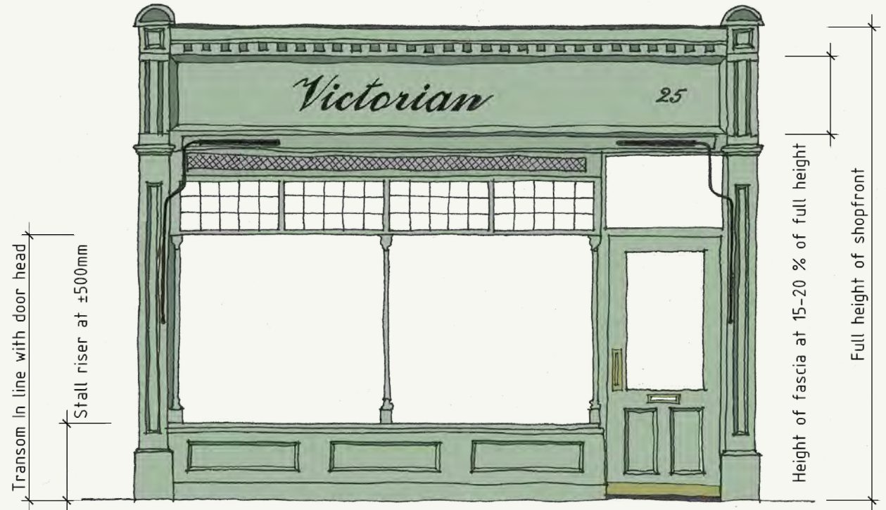
Shown above are some general, recommended proportions for shopfront design based on local precedent.
